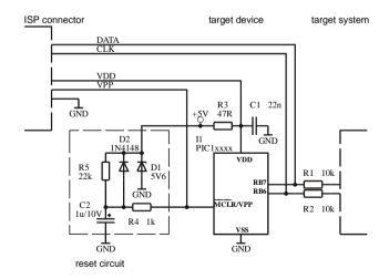
**Note:** External reset circuit is necessary only if VDD power-up slope is too slow.
